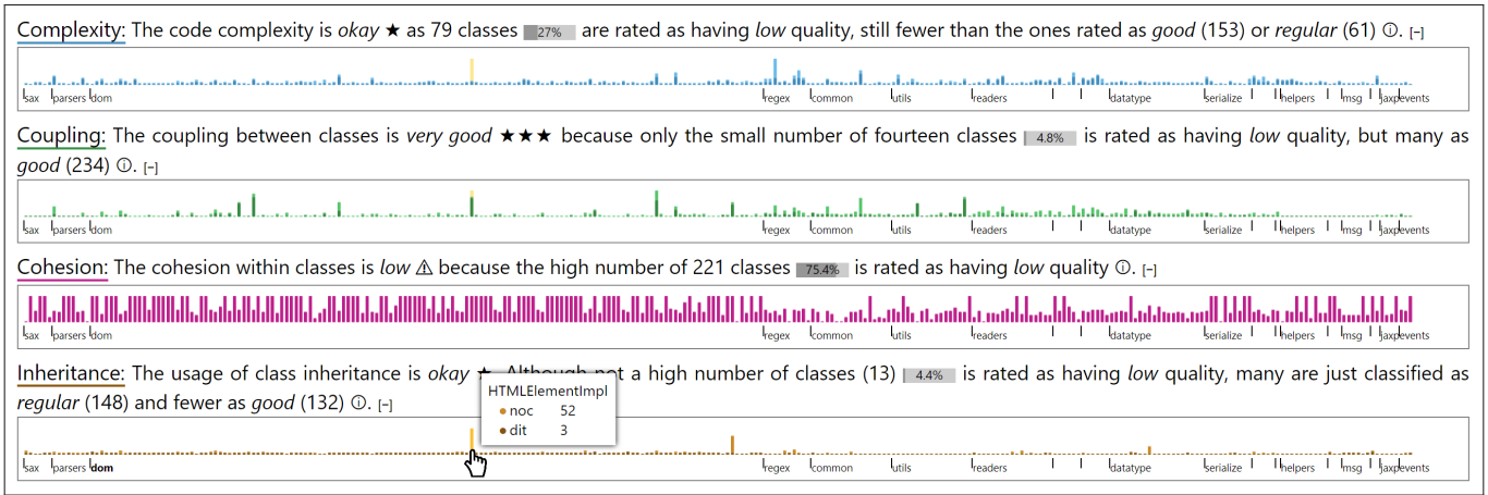
Fig. 7. Low quality in HTMLElementImpl found through active exploration of the embedded detail visualizations of coupling, cohesion, and inheritance.
