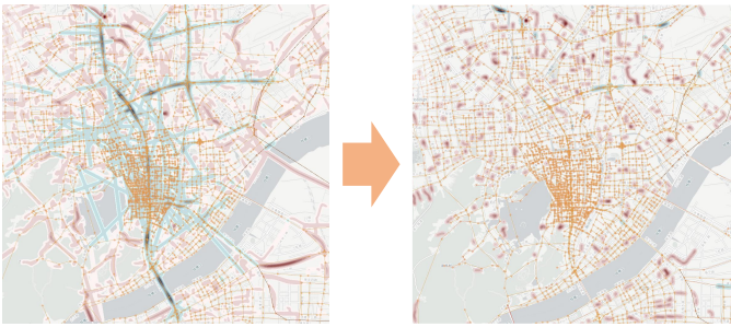
Fig. 13. (Left) Without cleansing and parameter adjustment the map matching underlies many candidate errors (red) as well as path length errors (blue). (Right) After the iterative adjustment (Iteration 9), the map view shows much fewer errors.
