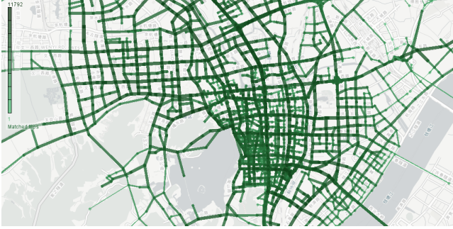
Fig. 6. The matched trips overlay gives information where and how many trips were matched. This is double-encoded by edge thickness and color. Because of the highly varying amounts of matched movements a log scale is used.
