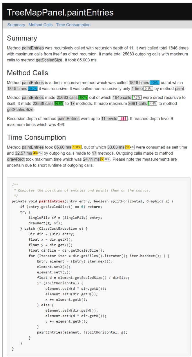
Fig. 1. Execution report for the method TreeMapPanel.paintEntries of a program that draws a treemap visualization for a file hierarchy encoding file sizes in the size of the nested boxes.
